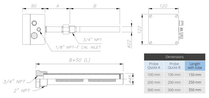
**Quote A** can be set to withdraw the probe head (with electronics inside) from hot external surface of the duct **Quote B** is the insertion length into the duct
