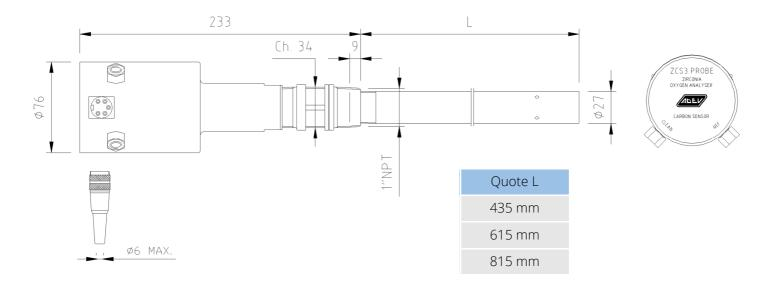
ZCS Carbon Probe, located directly in the furnace heat zone, responds almost immediately to changes in the carburizing atmosphere and totally eliminate the need for gas sampling system
